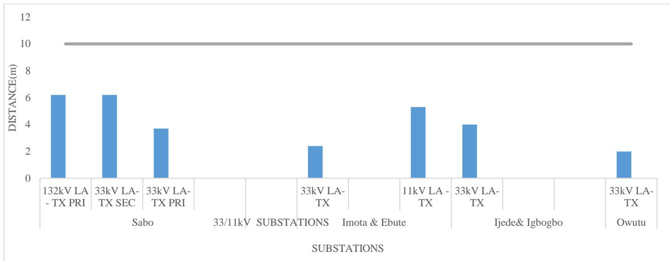
Fig. 12: Measurements of Lightning Arrester Distance to Transformer on 132 kV-11kV Ikorodu Substation
