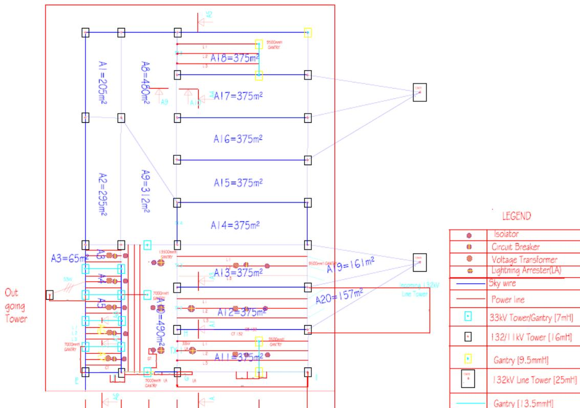
Fig. 3: Plan View of Ikorodu 132/33 kV Substation, showing Mesh Area of Ikorodu Transmission Substation Using Mesh Method
