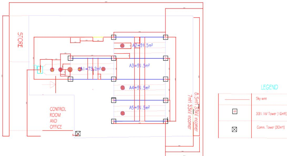
Fig. 2: Plan View of Imota, Ikorodu 33/11kV Substation, showing Mesh Method of Screening Substation Elements Typical to Ijede, Ebute and Igbogbo Substation
