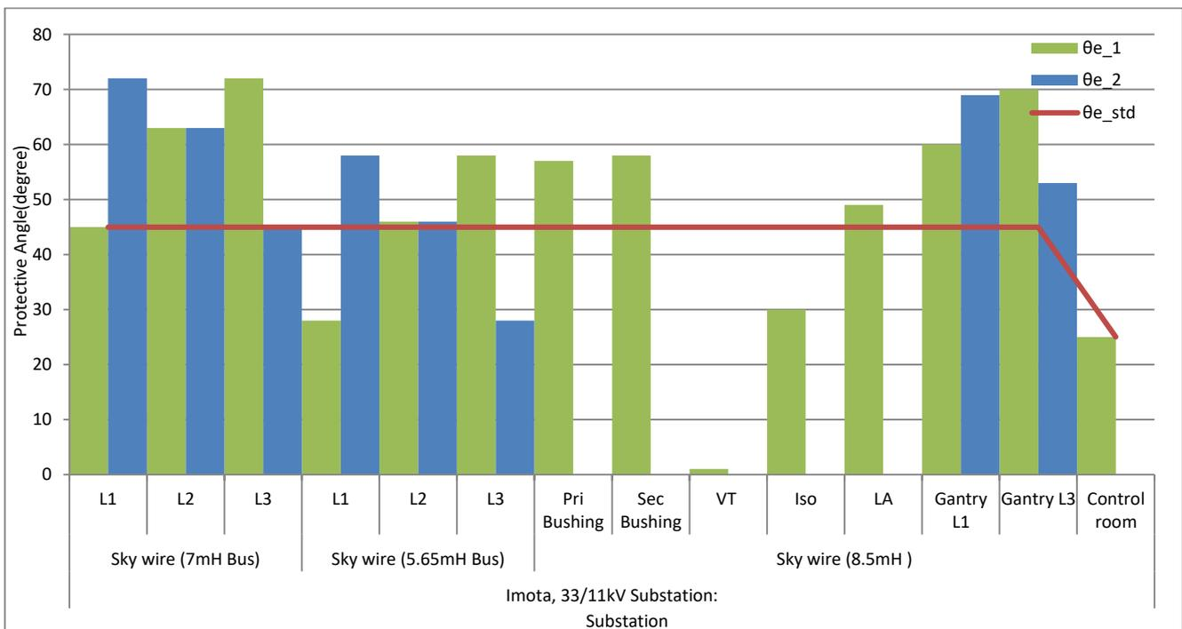
Fig. 5: Measurements of protection angles with respect to standard provided by adjacent OGWs 1and 2 for 33/11kV Imota, Ikorodu Substation -Sky wire
