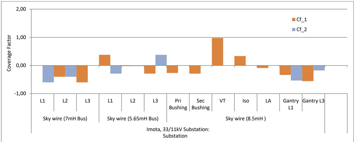
Fig. 9: Coverage factors from adjacent OGWs 1 and 2 for each protected installation in 33/11kV Imota Substation, Ikorodu - Sky
