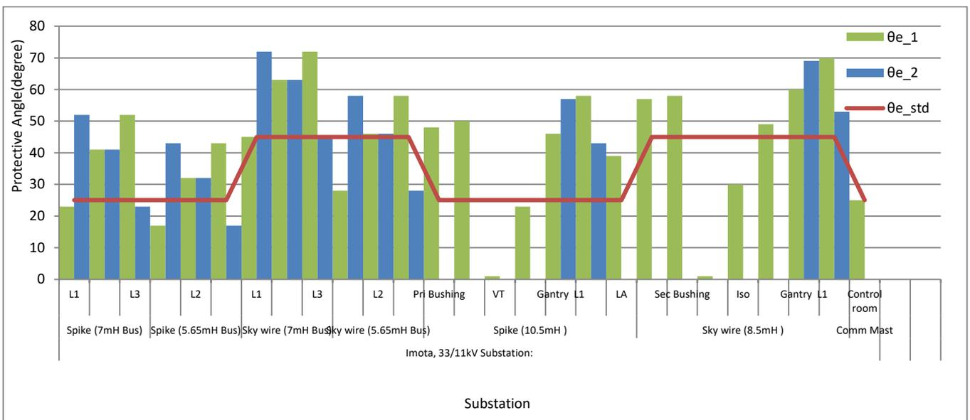
Fig. 7: Measurements of protection angles with respect to standard provided by adjacent OGWs 1 and 2 for 33/11kV Imota Substation -Sky and Spike
