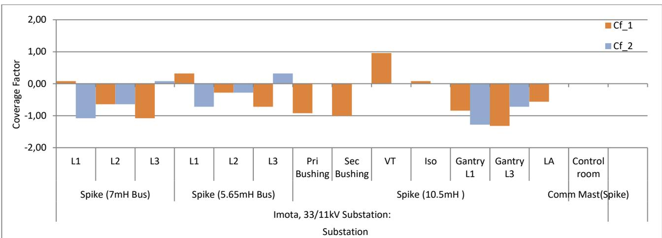
Fig. 10: Coverage factors from adjacent OGWs 1 and 2 for each protected installation in 33/11kV Imota Substation, Ikorodu – Spike
