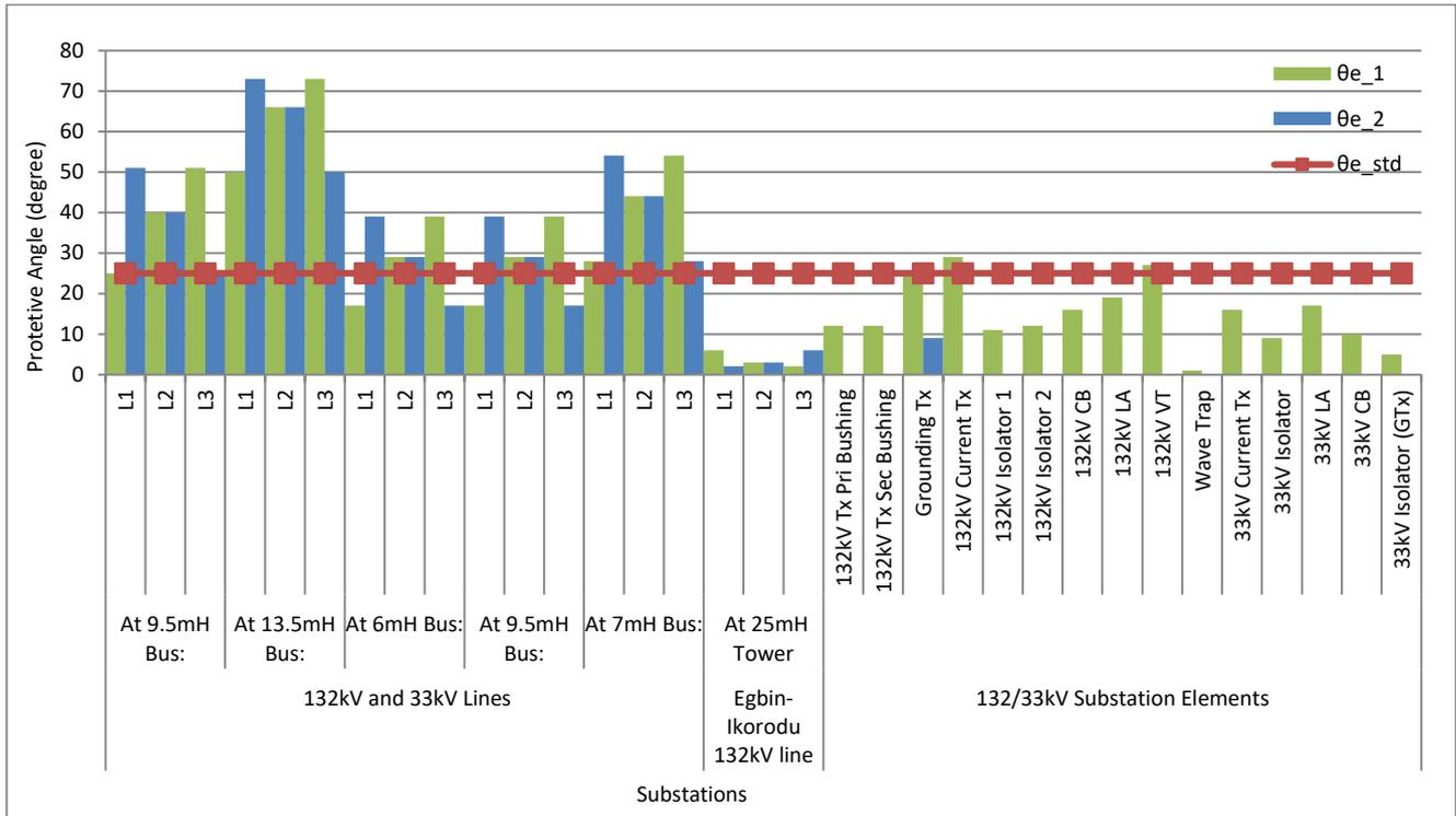
Fig. 4: Measurements of protection angles with respect to standard provided by adjacent OGWs 1and 2 for 132/33kV Ikorodu Substation
