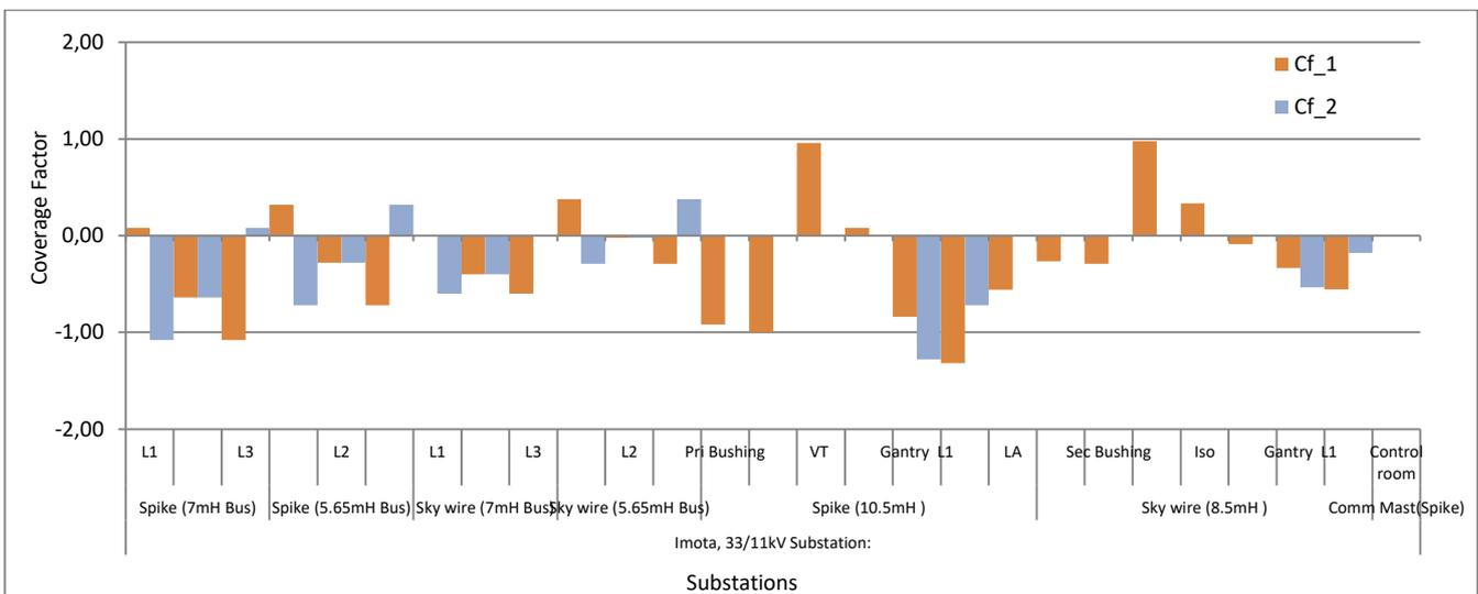
Fig. 11 Coverage factors from adjacent OGWs 1 and 2 for each protected installation in 33/11kV Imota Substation, Ikorodu - Sky and Spike
