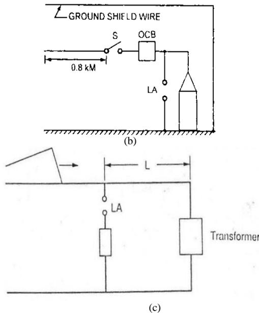
Fig. 1: (a) Protective Angle Method, (b) Shielding method, (c) Location of Lightning Arrester to Transformer (Adapted from [5] [12] and [7] respectively)
