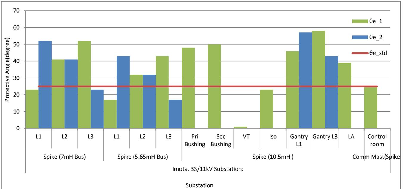
Fig. 6: Measurements of protection angles with respect to standard provided by adjacent OGWs 1 and 2 for 33/11kV Ikorodu Substation –Spike wire
