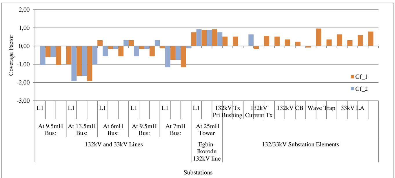
Fig. 8: Coverage factors from adjacent OGWs 1 and 2 for each protected installation in 132/33kV Ikorodu Substation – sky
