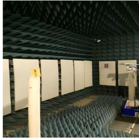
Fig. 9. Antenna under test in the anechoic chamber.
