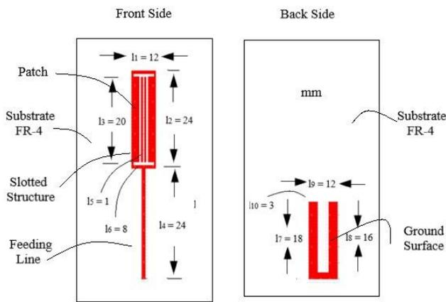
Fig. 3. Designed antenna structure.
