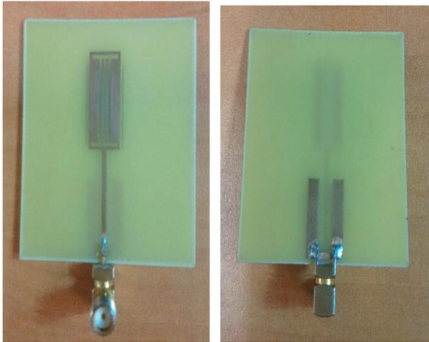
Fig. 6. Prototype antenna, front and back side respectively.
