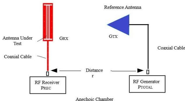
Fig. 8. Measuring technique configuration.
