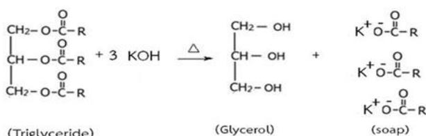
Fig. 8. Typical reaction involved in soap preparation
