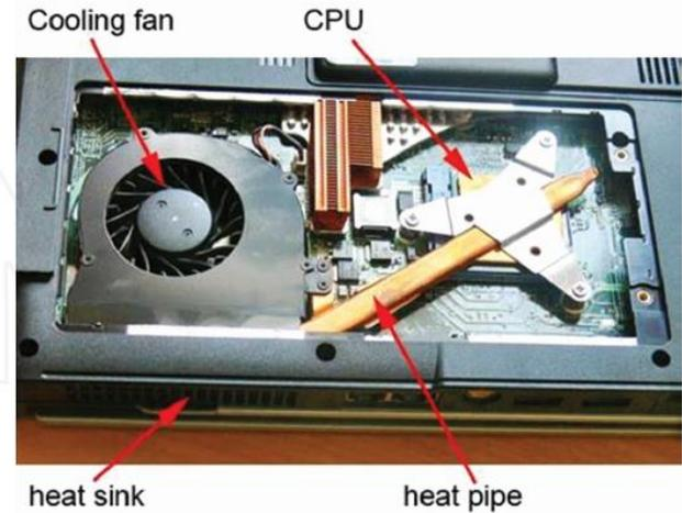
Fig. 6. Heat sink with fan and heat pipe for laptops cooling [6], [17].
