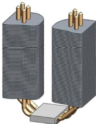
Fig. 5. Heat sink with heat pipes for desktop computer cooling [6], [8].
