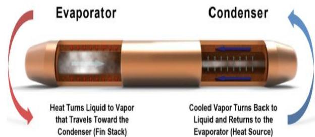
Fig. 3. Cylindrical heat pipe structure [15].
