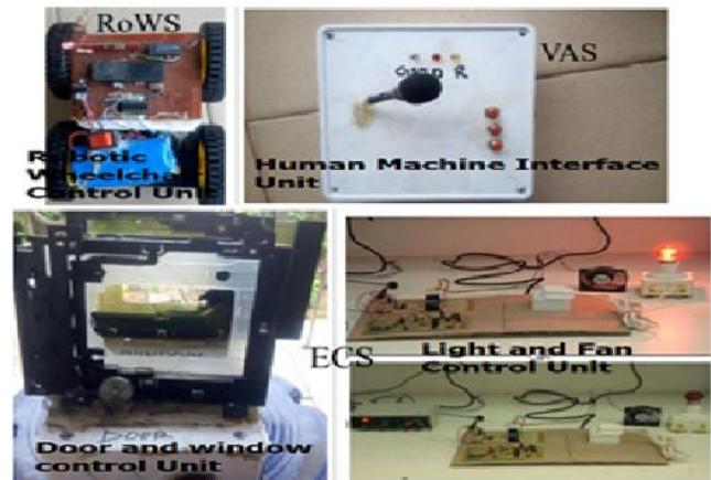
Fig. 5: The full smarthome system showing the VAS, ECU and the RoWS
