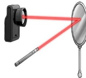
Fig. 3. A laser beam has been reflected by the mirror (placed at the right from the laser) and acts with an electromagnetic radiation pressure on the mirror directed towards to the right.
