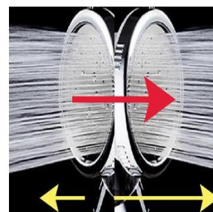
Fig. 8. The left hand has been placed in the waterjet emitted towards to the left and the right hand has been placed in the waterjet emitted towards to the right. The resulting force has been oriented towards to the Right.
