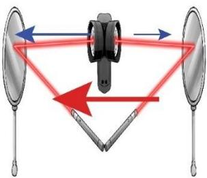
Fig. 10. The left mirror has been placed in the laser beam emitted towards to the left and the right mirror has been placed in the laser beam towards to the right. The resulting force has been directed towards to the Left.
