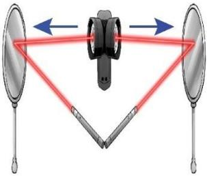
Fig. 9. Two lasers, pointing in opposite directions, emit two laser beams pointing in opposite directions. The left mirror has been placed in the laser beam emitted towards to the left and the right mirror has been placed in the laser beam towards to the right
