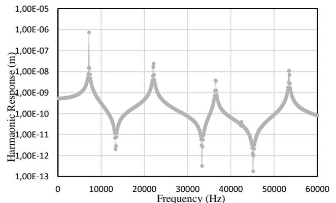
Fig. 3. Frequency response for Al-St-Ad-Al-St arrangement
