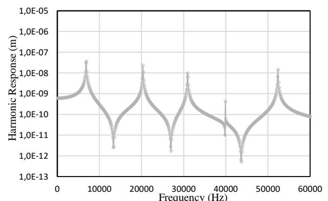
Fig. 4. Frequency response for Al-St-Ad-St-Al arrangement
