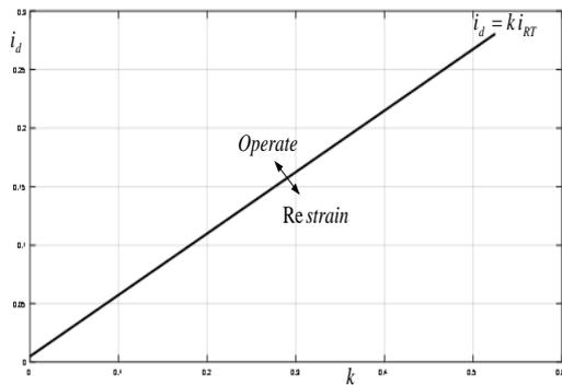
Fig. 5. Operating diagram of biased differential scheme
