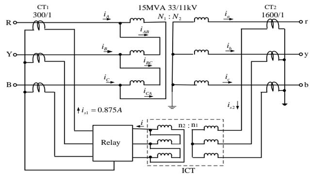
Fig. 17 Ratio correction and phase-angle correction using one set physically-connected ICT
