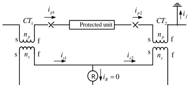
Fig. 3 External fault
