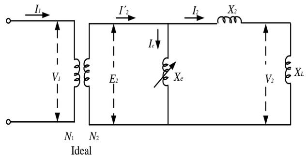
Fig. 6. CT equivalent circuit
