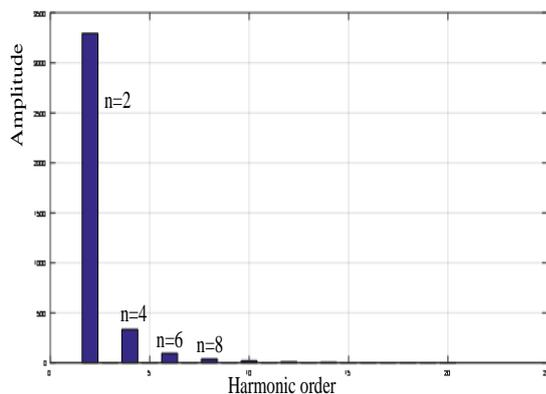
Fig. 14 magnetizing inrush current harmonics
