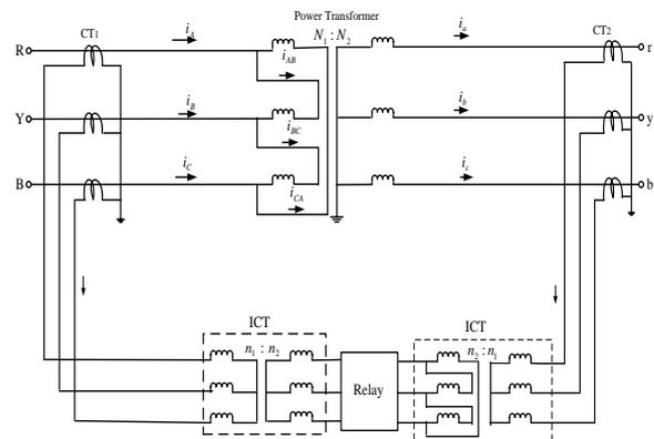
Fig. 18 ratio and phase-angle correction using two sets physically-connected ICTs
