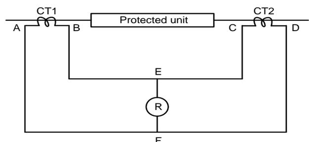
Fig. 1. Current differential protection
