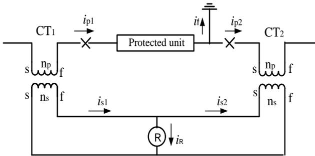
Fig. 2. Internal fault
