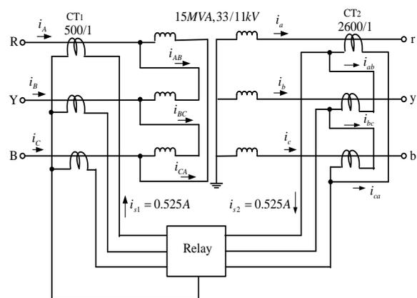
Fig. 16 ratio and phase-angle correction by delta connection of line CTs
