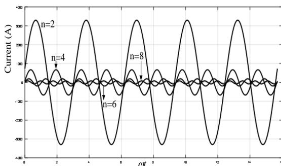
Fig. 15 magnetizing inrush current harmonics
