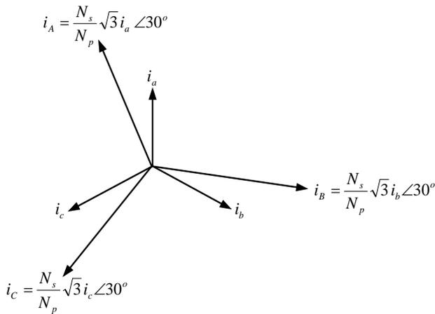
Fig. 10 Primary and secondary currents phasors for steady-state operation.
