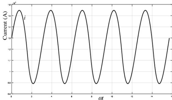
Fig. 13 magnetizing inrush current waveform
