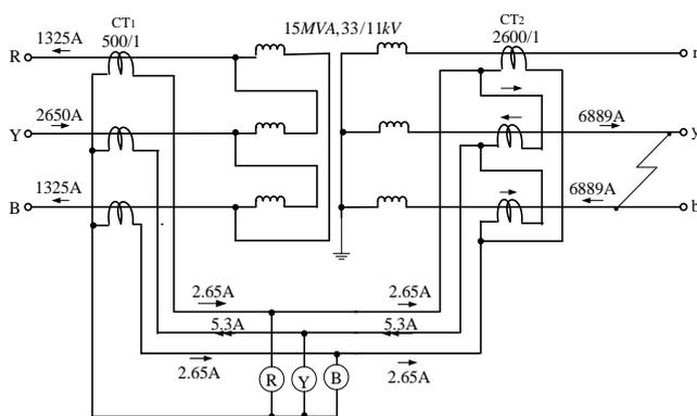
Fig. 20. Current distribution under phase-to-phase through fault condition
