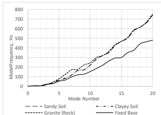
Fig. 3. Frequency versus Mode Number for Various Foundation Soil Types.
