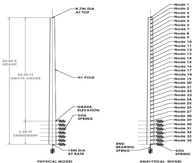
Fig. 2. Soil Embedment for a Class H1 utility tapered wood pole and Finite Element Analytical model.
