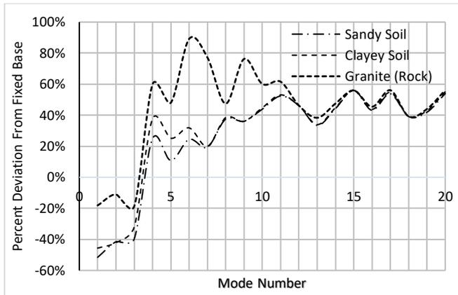
Fig. 4. Frequency Deviation Vs Mode Number for Various Foundation Soil Types.
