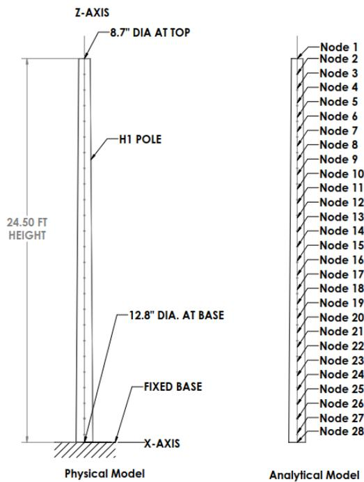
Fig. 1. Fixed base model for a Class H1 utility tapered wood pole and corresponding analytical model.
