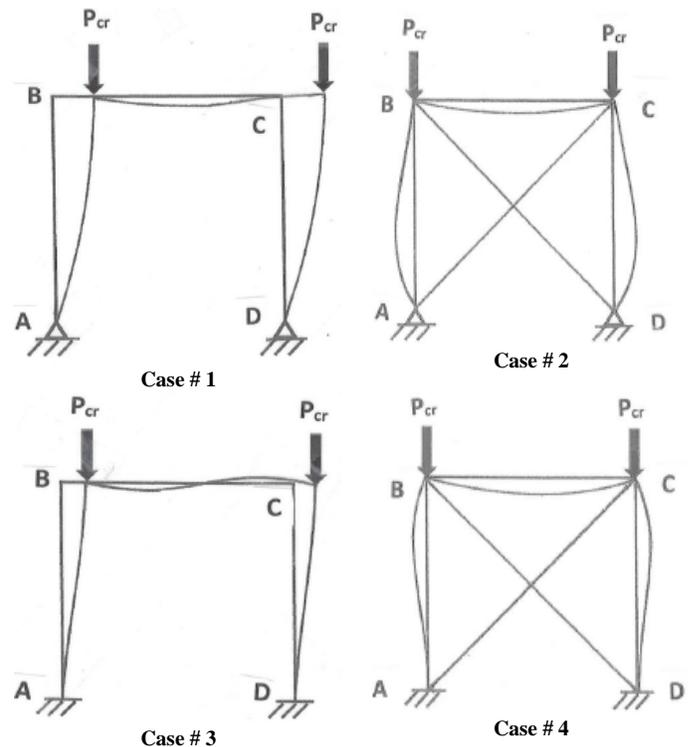
Fig. 1. Unbraced and braced frames with columns either pinned or fixed at the base.
