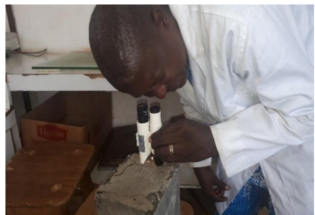
Fig. 5. Crack measurement with microscope.
