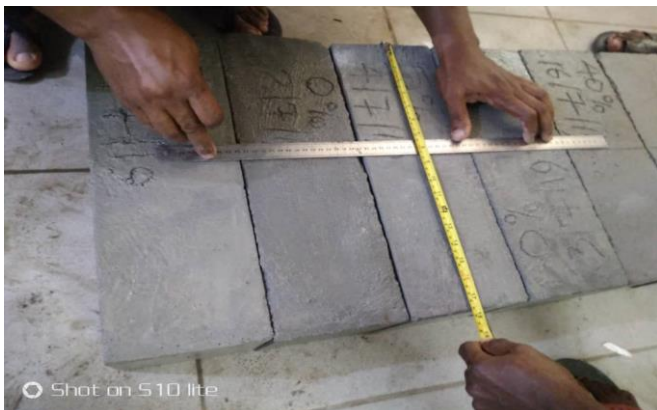
Fig. 3. Measuring the sample beams.
