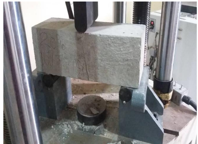
Fig. 4. Crushing of beam showing the first crack.
