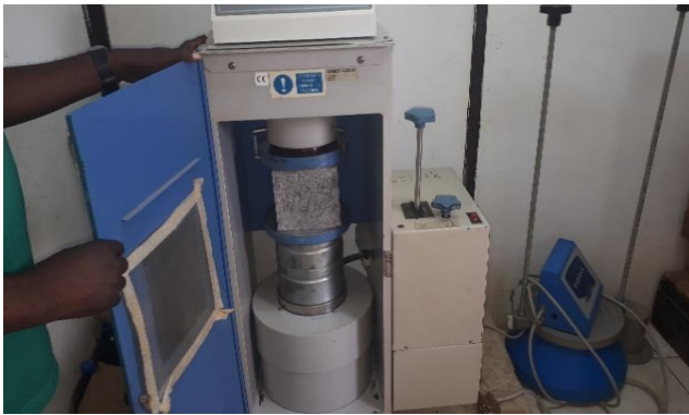
Fig. 2. Compression of cube sample.
