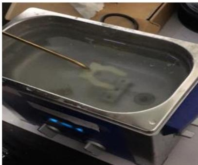
Fig. 14. Gripper heat actuation through hot water.
