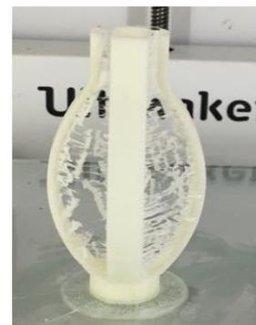
Fig. 9. First prototype of gripper having string like structures.
