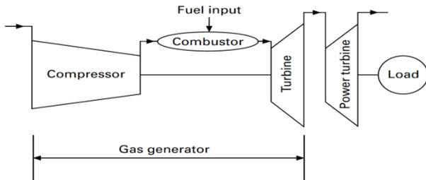
Fig. 1. Industrial gas turbine engine layout.
