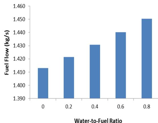
Fig. 4. Fuel flow against water-to-fuel ratio.
