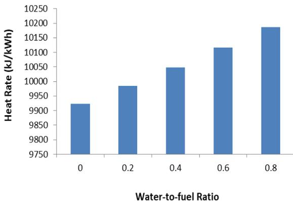
Figure 5: Heat Rate against water-to-fuel ratio.
