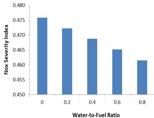
Fig. 3. Nox severity index against water-to-fuel ratio.
