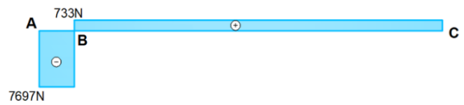
Fig. 5. Shear force diagram of the bead breaker arm and pry bar assembly.
