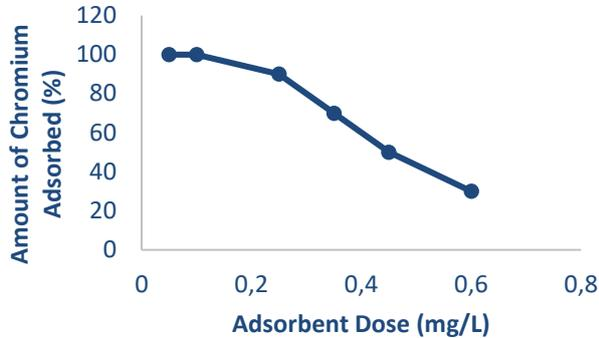
Fig. 3. Chromium Adsorbed versus Adsorbent concentration.
