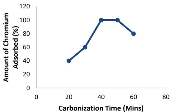
Fig. 2. Chromium Adsorbed versus Carbonization Time of yam Peel.
