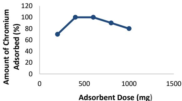
Fig 4. Chromium Adsorbed versus Adsorbent concentration for Activation before Carbonization.
