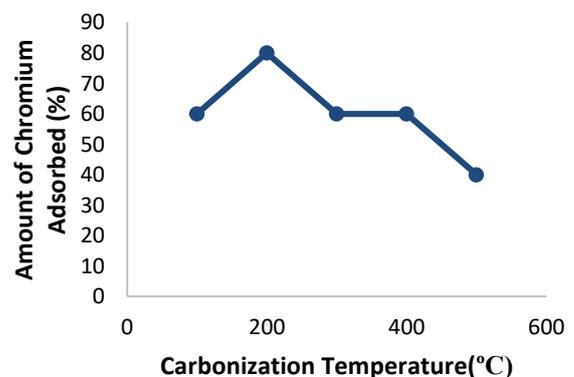
Fig. 1. Chromium Adsorbed versus Carbonization Temperature of Yam Peel.
