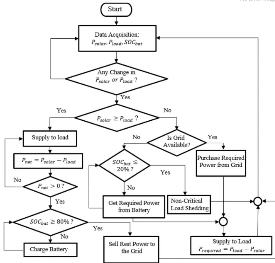
Fig. 6. Flowchart of the proposed algorithm for the grid connected PV system
