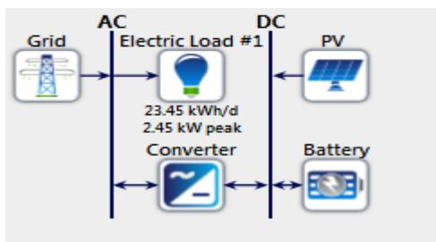
Fig. 5. Complete model of a grid connected PV power system
