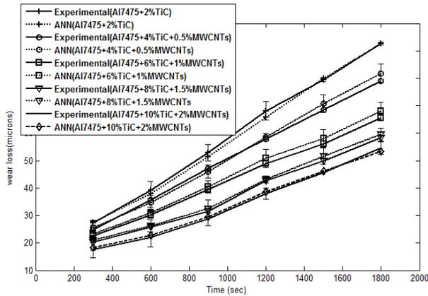
Fig. 6. Experimental vs. predicted values of wear loss as a function of time
