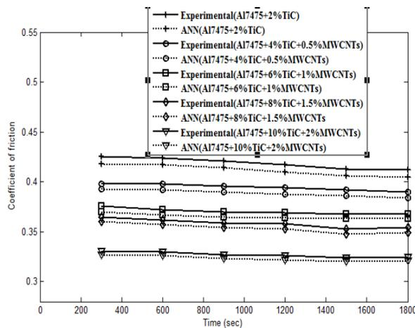
Fig. 7. Experimental vs. predicted values of Coefficient of friction as a function of time.
